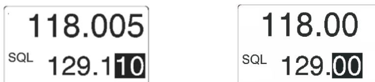
8.33 kHz channel spacing (left) / 25 kHz channel spacing (right)
