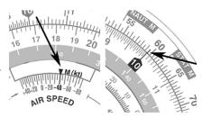
With the scales set as in the above example, conversions of TAS to Mach Number can be made.
