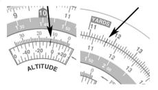
The Density Altitude is a very important issue for the interpretation of the performance tables in the aircrafts flight manual. Data in the table is based on ISA conditions at the present temperature at the altitudes indicated.
