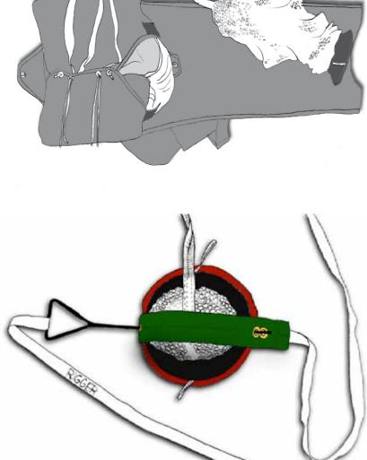
Note! Locking rod and strap should be at 90° angle to closing loops.
