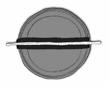
**Rigger Tip:** Once you have cut the first hole in the Spandura® for your loop to come through, fold the cap perfectly in half at that hole, making a crease. Unfold the cap, and you can see just where 180° is and where your other hole should go.
