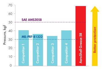
A step change in extreme-pressure protection. AeroShell Grease 58 has better load wear protection compared with MIL-PRF-81322 greases in ASTM D2596 tests.
