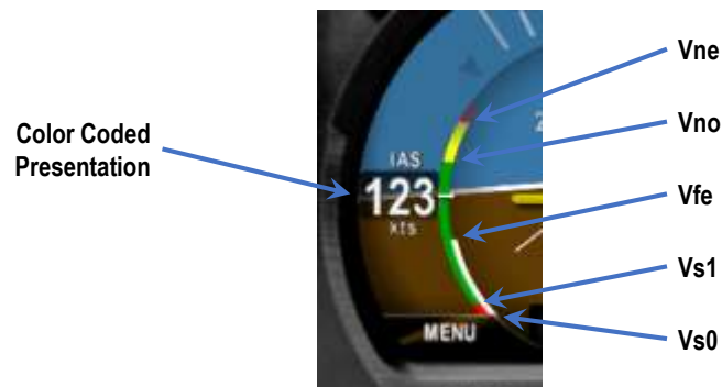
Figure 15 - AI Mode, V-Speed Limits
