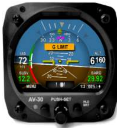
Figure 29 – Example of Alert Annunciator on Screen
