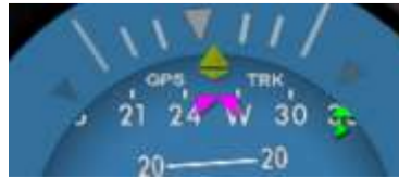
Figure 16 - AI Mode, Direction Indication, Bearing To Off-Screen
