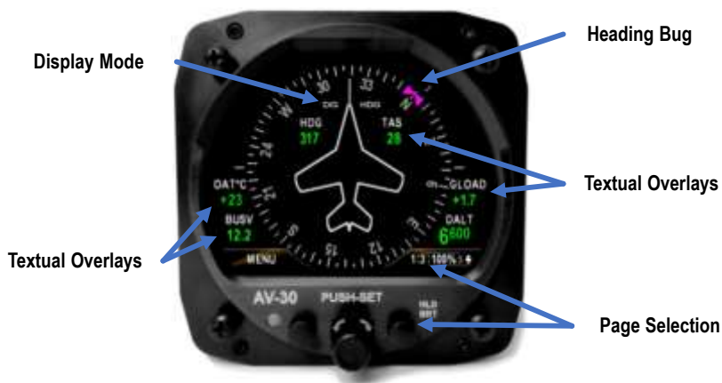
Figure 23 – Basic DG Mode User Interface
