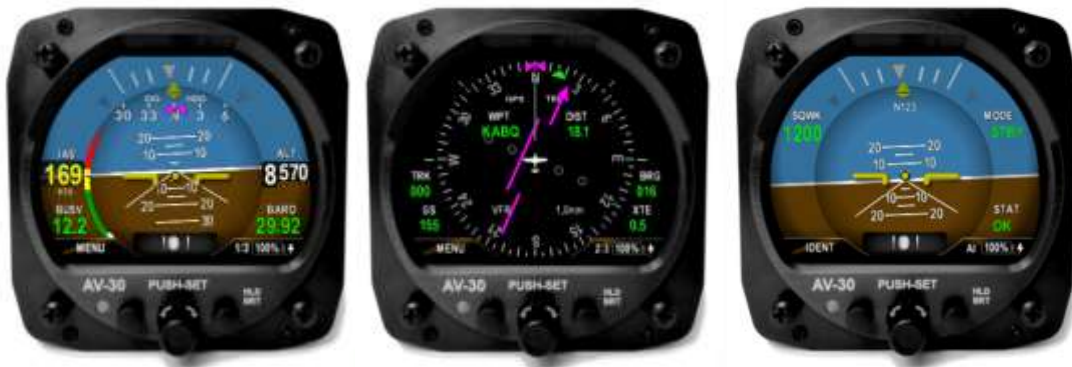
Figure 1 - AV-30-C Multi Mode AI/DG/Transponder – Basic Display
