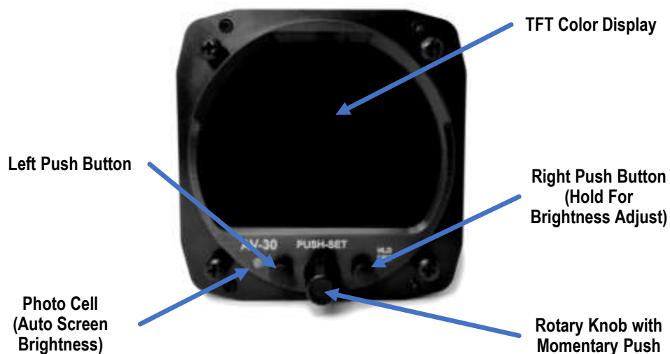
Figure 5 - Common User Interface Components
