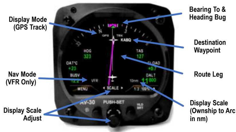
Figure 25 – GPS ARC Mode
