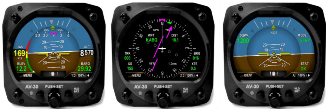
Figure 1 – AV-30-C Multi Mode AI/DG/Transponder – Basic Display
