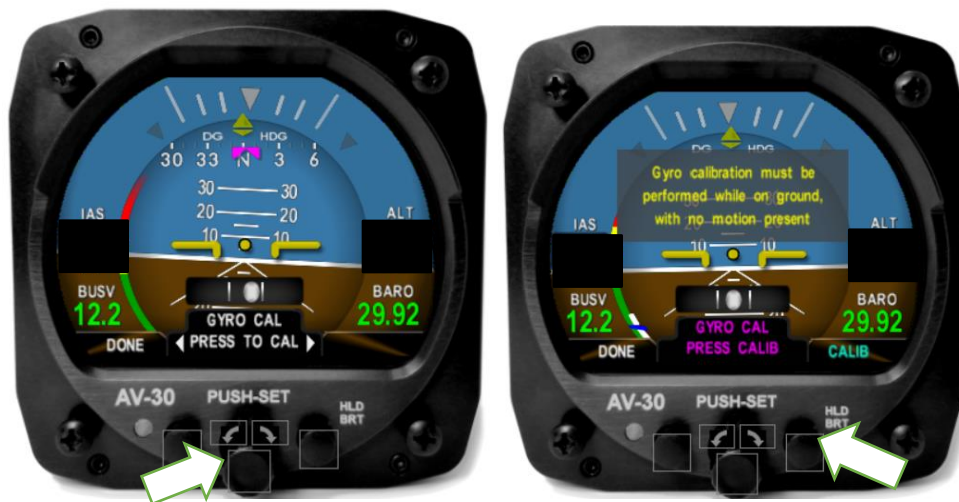
Figure 30 - Gyro Calibration Selection
