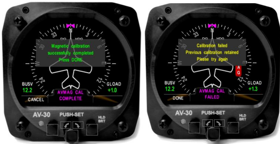
Figure 39 – AVMAG CAL Success and Failure Screens
