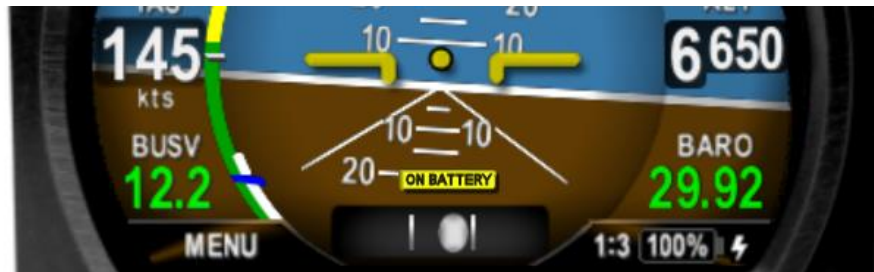
Figure 44 - On Battery Operation
