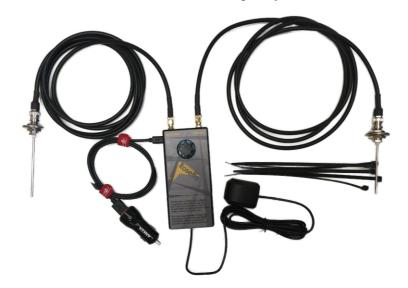
Connect the assembled system to a suitable USB source 5.2V 2.1A using the power lead provided.
