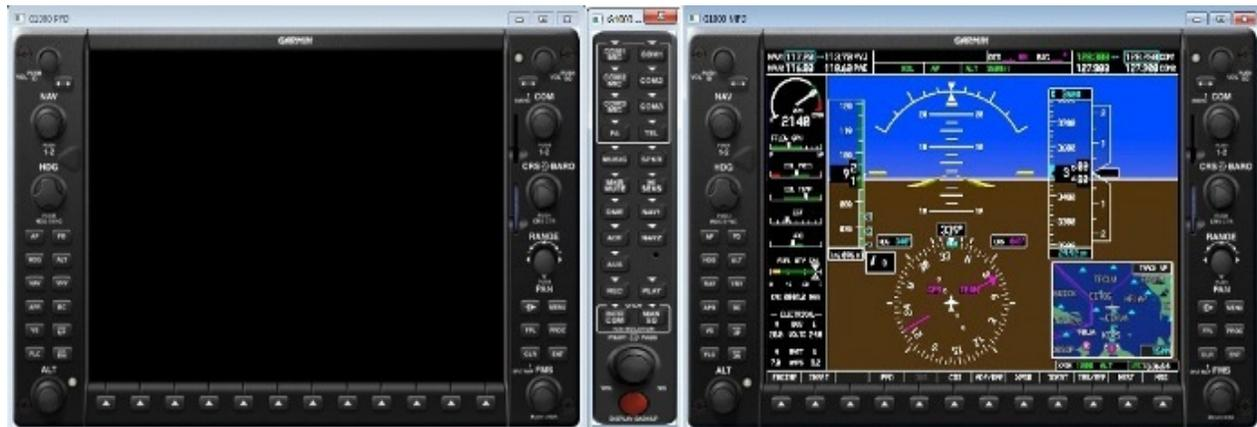
In the airplane, you can only simulate Reversionary Mode by manually dimming one display, and manually switching both displays to Reversionary Mode by pressing the red Display Backup button on the audio panel. What the student sees (the primary flight instruments and engine data on both displays) is realistic, but manually setting up Reversionary Mode like this provides a far less realistic training experience than generating a spontaneous display failure from VISPRO.
