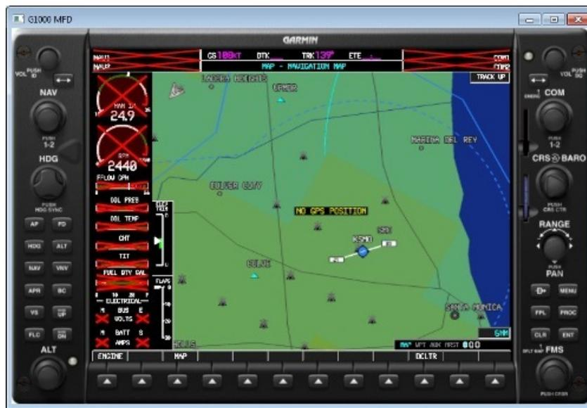
VISPRO, the native IOS for P3D based simulation, lets you control the simulation's environment, change the weather, reposition the student's aircraft, and trigger malfunctions ... all in real time as the simulation is running. It gives you professional-quality tools for monitoring, instruction, and analysis.
