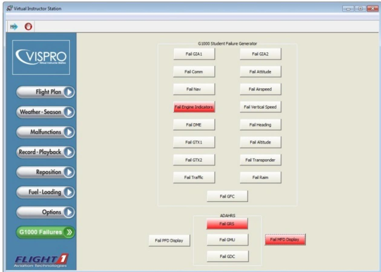
The G1000 Failures selection, allows the instructor to fail the following Line Replaceable Units (LRUs) and individual components:
