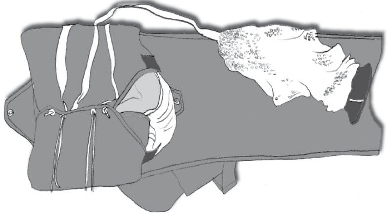
Stand the pilot chute upright on the locking strap. While compressing pilot chute, neatly and symmetrically tuck the pilot chute's canopy cloth in between the coils of the spring. Continue until the pilot chute is fully compressed and lock with locking strap.
