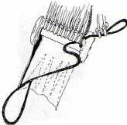
Position white mark on the control at the connector link. Form loop, pass through lines 1 & 2 and/or 23 & 24.
