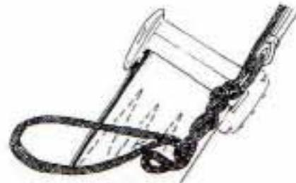
Secure last braid loop to loop handle with rigger's seal thread (4 lbs).
