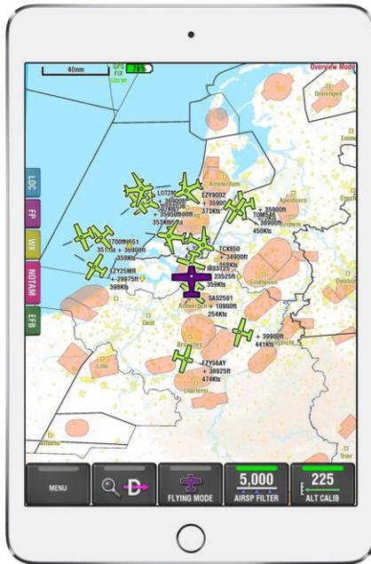
Altitude must be pre-flight cross-checked by comparing the aircraft's altimeter with the GPS altitude displayed on the EFB application.
